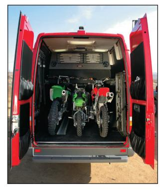
**Loads of space for bikes and support equipment.** The walls and floor have a tough coating -- just hose it out. A high-end sound system was also installed.
